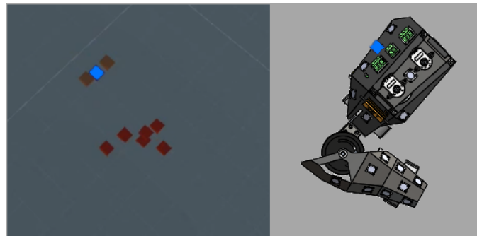
Figure 12: Sensor tracking in the virtual environment compared to the orientation of the physical device. One sensor is highlighted to show its position on the physical device.
